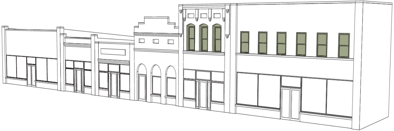
Although Mount Pleasant's downtown has a few two-story buildings, the patterns of windows create a rhythm of openings along the street wall.
